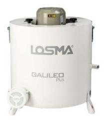
to 2,750 m3/h, Galileo technology combines **static and dynamic filtration** to ensure maximum efficiency. It is equipped with a new turbine that aspirates oil mists and polluting particles in the air, which join together and return to the liquid state due to centrifugal force. Before being returned to the environment, the air passes through a new multilayer filter capable of retaining even the smallest particles.
