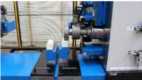
Fig. 1 – 2 Horizontal Trimming-Beading Machine R400-I for tubes 300 – 2000 mm length
