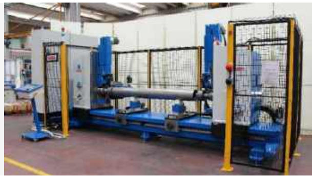
Fig. 1 – 2 Horizontal Trimming-Beading Machine R400-I for tubes 300 – 2000 mm length
