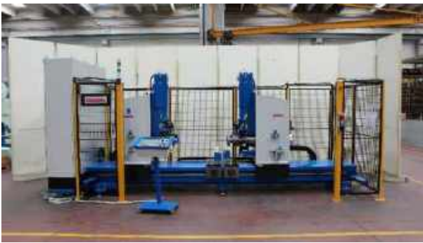
Fig. 1 – 2 Horizontal Trimming-Beading Machine R400-I for tubes 300 – 2000 mm length
