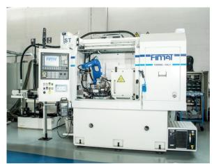
In order to get the required result, the grinding wheel slide is driven by a linear motor controlled by a high resolution absolute scale, thus granting the high dynamic and precision required by the process.
