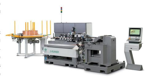
capable of processing tubes up to 35 mm diameter was developed. It has been integrated into a flexible manufacturing cell consisting of an automatic handling system to unload the parts from the 3-RUNNER and load them on to the E-TURN32 bending machine. The E-TURN32 is an All-Electric CNC tube bending machine capable of in-process RHS and LHS bending. The E-TURN32 not only bent the part but also
