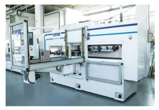
The racks slides are driven by Planetary Roller Screws, Torque Motors and High Resolution Absolute Encoders. The motors are directly connected to the screws as well as the encoders, in order to avoid any backlash due to elastic joints and to ensure the high precision required for the NC synchronization of the slides.
