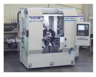
The machine can be set up just for hard milling or for soft+hard milling capabilities. For each set up, one or two workheads can be assembled depending on the required cycle time.
